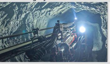
Adopting high efficient and fast electro-proportional hydraulic control drilling system, including automatic drilling, automatic retraction, automatic release of jamming brazier and other functions.
